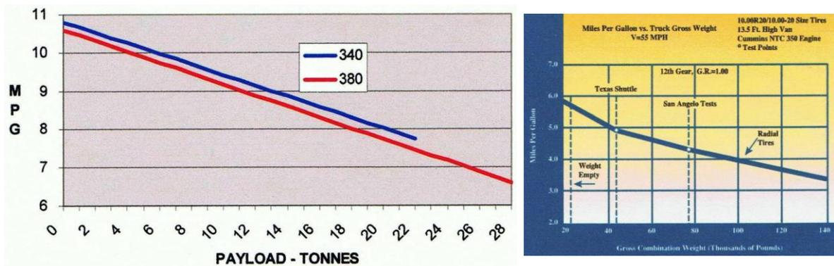
Figure 3.1-5: Left - Regression lines for 340 and 380 Volvo FM12 tractors with the trailers of variable payload from Coyle (2007); right – Good Year Testing Data reproduced from Good Year (2008)
