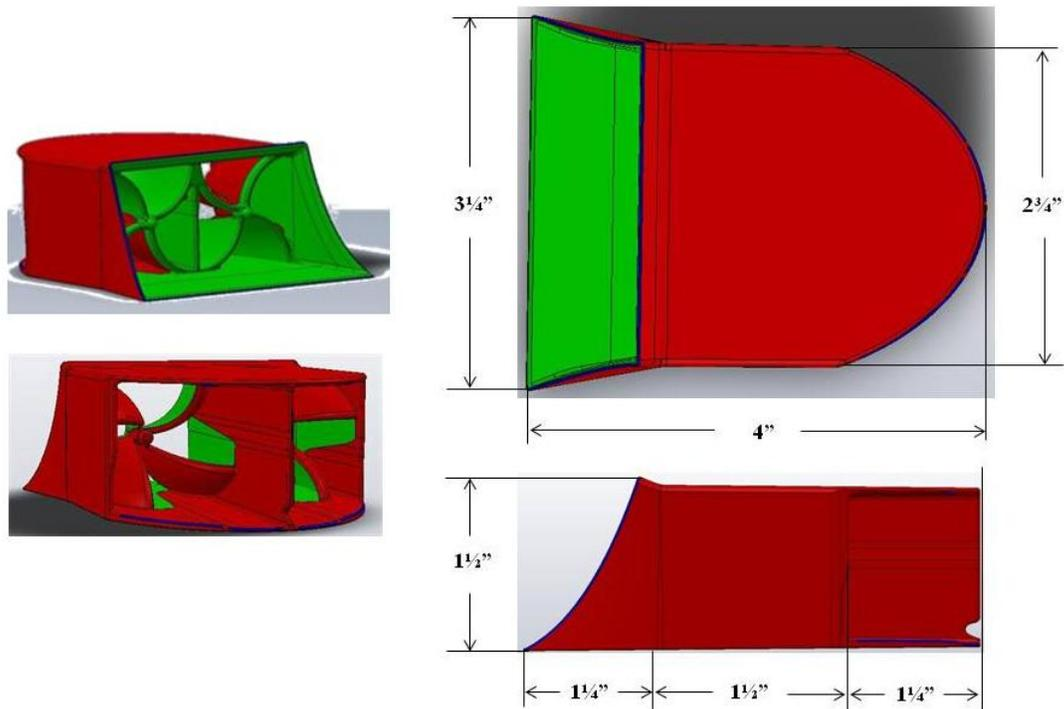
*Figure 3.2-1: Left - Prospective front and rear views of VorBlade as in Figure 2.1-5; and right – external dimensions of the VorBlade vortex generator*
