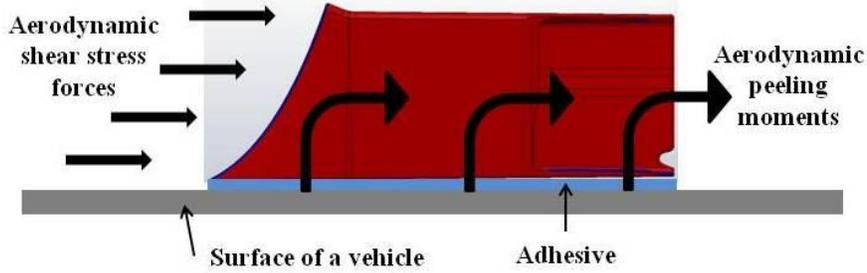
Figure 3.2-2: Schematic of distributed aerodynamic shear stress forces and peeling moments acting on VorBlade generator and adhesive
