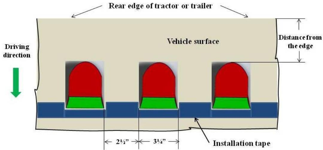
Figure 3.2-4: Schematic of the installation masking tape with the indentation-marked locations for VorBlade generators on the rear edges of tractors and trailers
