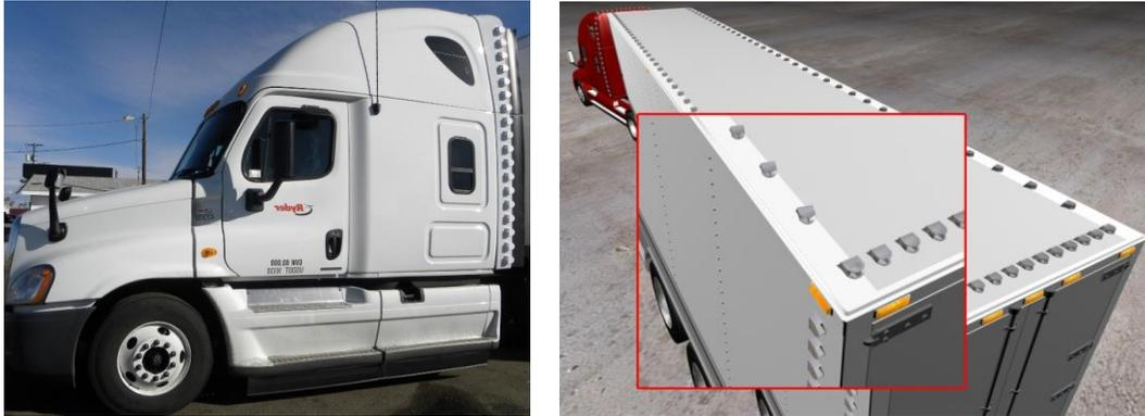
Figure 3.1-4: Closer look at VorBlade vortex generators on a driver side of the test tractor and on the trailer roof
