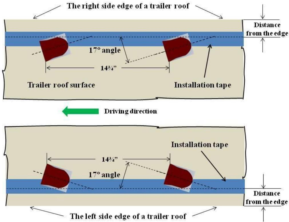
Figure 3.2-5: Schematic of the installation masking tape with marked locations for VorBlade generators on the side edges of the trailer roof
