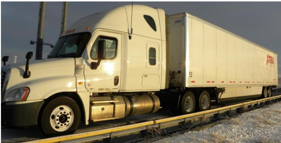
*Figure 3.1-1: The control vehicle on the weigh scales at the Tomahawk Auto & Truck plaza*
