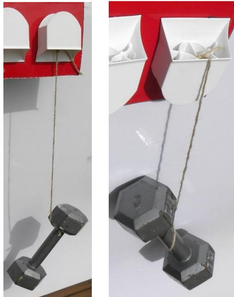
*Figure 3.2-3: Simple shear and peel tests of the two-sided adhesive tapes with 10 lb dumbbells*
