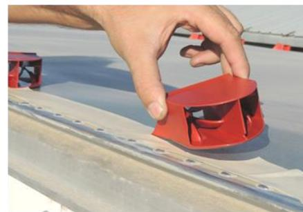
*VorBlade™ vortex generators must be positioned at 17 degrees to the roof side edges and the front of each generator must be oriented towards the trailer center line.*
