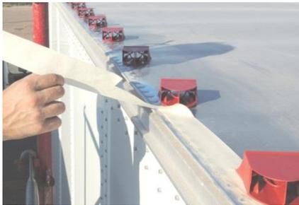
4a: Remove installation template from the trailer.
